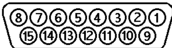
DB-15 Male wiring side
