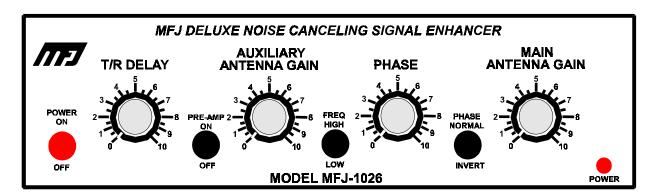
**POWER ON/OFF:** This switch turns the main power off and on. In the OFF (out) position, the MFJ-1026 is bypassed. The RADIO and MAIN ANTENNA connectors have a direct connection between each other whenever power is removed or this switch is turned off.
