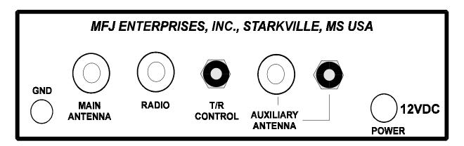
**GND:** This connection is used to connect the MFJ-1026 to the station ground buss. Always use a short ground wire when making this connection. Always try to use solid copper wire (not braided wire) when making a ground connection. Woven or braided wire has higher RF resistance than solid conductors.
