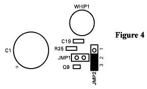
When the pre-amp is used with the external antenna (Figure 3 & 4) we recommend removing the internal telescoping antenna (WHIP) to ensure reception isn't compromised.
