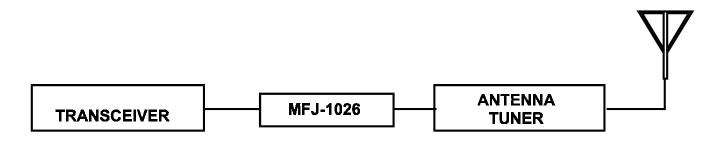
When using an amplifier install the MFJ-1026 between the transceiver and the amplifier input. NEVER install the MFJ-1026 on the output of either an amplifier or antenna tuner!
