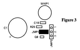
For moderate sensitivity, JMP2 must be activated. To activate JMP2 remove the shorting clip from previous position and place it across pins 2 and 3 of JMP2 (see Figure 4).
